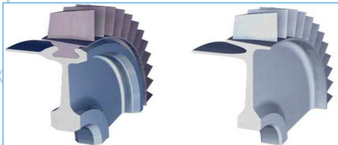
Left: Traditional blade/disk assembly. Right: New BLISK component
